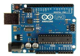
Arduino boards are able to read inputs - light on a sensor, a finger on a button, or a Twitter message - and turn it into an output - activating a motor, turning onan LED, publishing something online.
